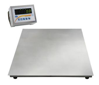
Calibratable stainless steel parcel scales up to 6,000 kg / Resolution from 0.1 kg/ Summing function / Tare weight storable / Piece counting function/ Limit value weighing Optional: analog output 4-20 mA, 0-10 V, OC switch contacts, RS-232, USB, LAN
